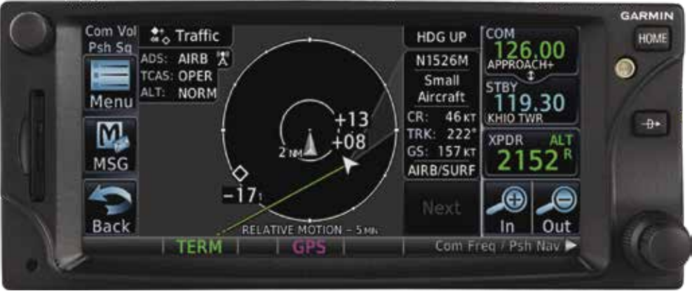
GTS series traffic alerts can be displayed on Garmin GTN 650/750 and 430W/530W series avionics
